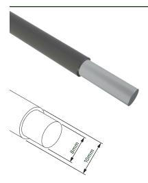
Kingsmill offers UV-stabilised **PVC Covered Solid Circular Aluminium** in a range of colours\*. Colours match the most common structural materials to reduce visual impact of a Lightning Protection conductor. Outer diameter (10mm) includes the PVC sheathing. Sold in the specified coil lengths only. **Use with 10mm clips.**
