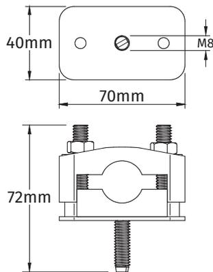
The **Insulated Lightning Conductor Cable Holder** is supplied with an M8 threaded stud.
