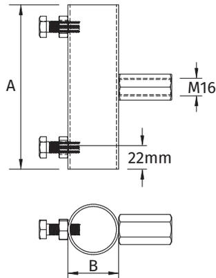
The **Air Terminal Mast Holders with Threaded Insert** are designed for use with our insulated and steel/insulated Air Terminal Masts.
