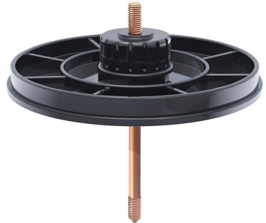
Kingsmill **Single Flange Earth Rod Seals** have been designed for use in concrete slabs with a nominal thickness of 300mm. They will withstand a pressure up to 80psi (5.5 bar) and have been tested accordingly.
