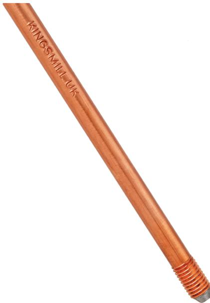
**Copperbond Earth Rods**, deep driven, usually provide the most cost effective earth system. They are made from a low carbon, high tensile strength (minimum 600n/mm<sup>2</sup>) steel core with a coating of 99.9% pure electrolytic copper, that has been molecularly bonded to the steel core.
