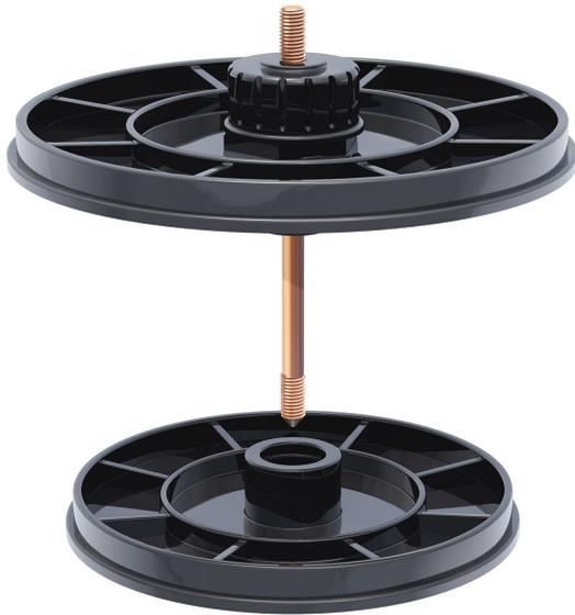
Kingsmill **Double Flange Earth Rod Seals** have been designed for use in concrete slabs with a nominal thickness of 300mm. They will withstand a pressure up to 80psi (5.5 bar) and have been tested accordingly.
