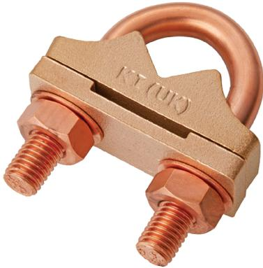
**Rod To Tape Type Clamps (U Bolt Double Plate Type)** join 25 x 3 conductor tape to the earth electrode/rebar without the need to drill the tape.
