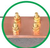
By using parallel fixings, the length of an Earth Bar can be significantly reduced. Also, parallel fixings can be used to accommodate cable lugs with two fixing holes.
